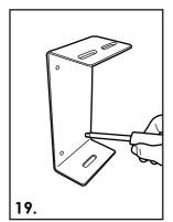
Align wall fixing bracket with drilled holes ensuring two slots are positioned at top and single slot at bottom. Screw 4 off 1.5" screws with washers (provided) into wall using a screw driver.
