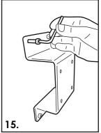
Alian wall fixing bracket with drilled holes and screw 4 off M5.5 x 50mm screws provided into wall using security allen key.
