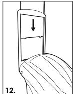
Place A4 sign behind clear polycarbonate sheet and slide into sign carrier so that lugs locate into slots along P.1 bottom of sign carrier.
