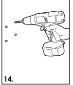
Using wall fixing bracket as template, mark out 4 off drill holes at top and bottom of bracket.
