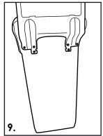
Open lid and position sign carrier at rear of bin so that the holes are aligned with holes in bin.
