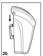
With the 3 off brackets already attached to the bin, hook the bin onto wall bracket so that the hooks locate into the slots.
