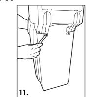
With lid open, install correct size sack (330mm x 533mm x 600mm available from Glasdon) by firstly hooking onto retention lugs at back of bin. in position.
