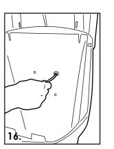
Holding bin up to wall bracket, place 4 off M6 x 16mm screws and washers provided through holes on inside of bin and fix with nyloc nuts using your fingers. Using a 10mm spanner and allen key provided tighten nuts until secure.
